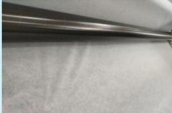
4. The shaped fibre mesh passes through the calendar and make the fibre web bond and finalize the design
