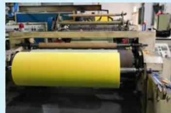
3. Compression of the two layers of non woven fabric while it is Cooling and make sure both layers can stick together closely. Rolling up the pressed non woven rolls and cut off the edges
