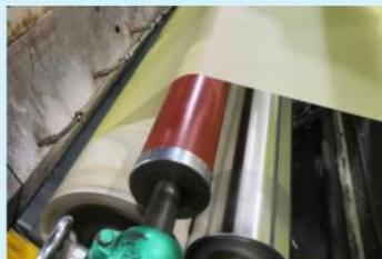
2. Extrusion the melt PE and coating it on the back fabric uniformly
