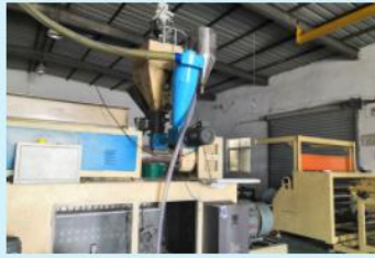
2. Polypropylene is conveyed to the inside of the machine body and melt
