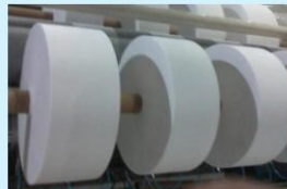
5. The non woven fiber web transferred to hot calender by net screen and will be high temperature pressed by hot calendar, rolling up, cut off the edges on both sides, eventually become a non woven roll.
