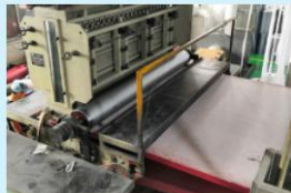
4. The stretched superfine fiber is transferred to the web former. Forming the embryonic form of non woven pp spunbond fabric.
